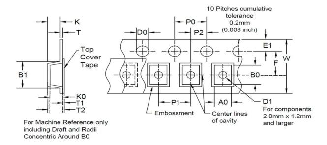
Note 1: B1 is for tape feeder reference only, including draft concentric about Bo.
